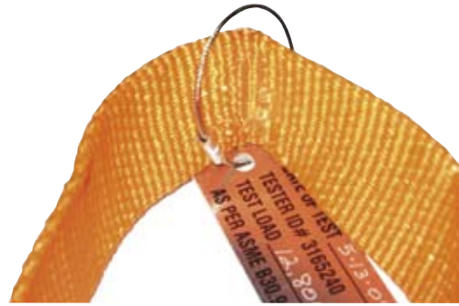
A wire and metal crimp was used to add additional information to this web sling. It damaged the eye before the sling was ever used.
